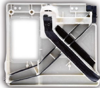
FIGURE 1 Part of a car seat backrest using E-LFT technology. The black endless fiber profiles are positioned both vertically and horizontally according to the load cases (© Weber Fibertech)
