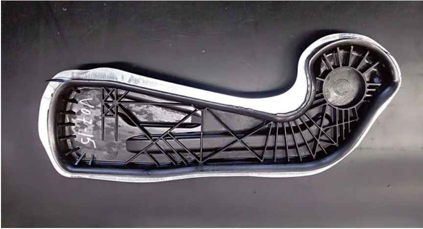
FIGURE 3 The transverse control arm as it leaves the press, untrimmed (© Weber Fibertech)
